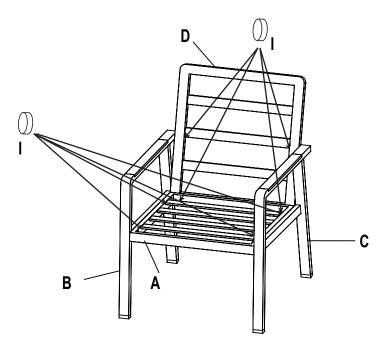
**STEP 5:** Tighten all the bolts on the chair and cover with the Plastic bolt cap (I). Turn the chair over and place the Seat cushion (F) and the Back cushion (E) onto the chair
