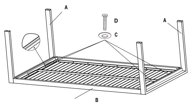
STEP 3: At the short side of Table top, using the M6x40 bolt (D) and Washer (C)
