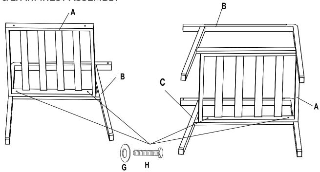
**STEP 1:** Attach Armrest 1 (B) to the Seat frame (A) using the M6x35 Bolt (H) and Washer (G)
