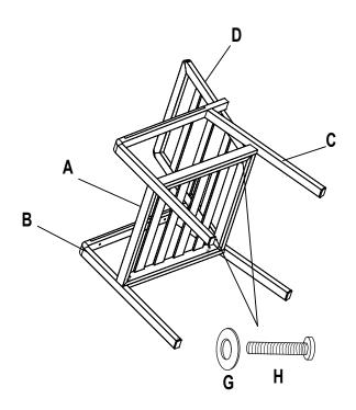
**STEP 3:** Attach Back board (D) to the Seat board (A) using the M6x35 Bolt (b) and Washer (a)
