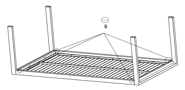
**STEP 4:** Tighten all the Bolts on the dining table and cover with the Plastic bolt cap (G), Turn the table over
