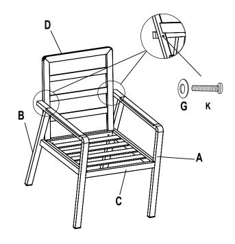
**STEP 4:** Attach Back rest (D) to the Armrest 1 (B) & Armrest 2 (C) using the M6x55 Bolt (K) and Washer (G)
