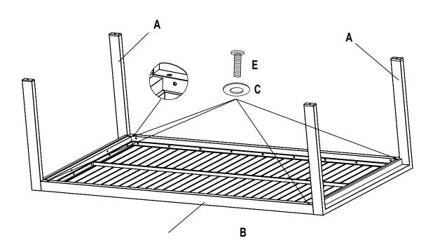
STEP 2: At the long side of Table top, using the M6x15 bolt (E) and Washer (C)
